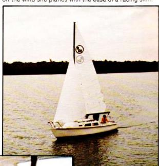
The weight and design of the RL-24 make it possible for it to be trailered with ease behind today's smaller cars. Since it draws only 12" of water, it can be launched almost anywhere. The lightweight aluminum spars can be raised or lowered in minutes on a hinged tabernacle; reducing the work load, and adding to the enjoyment of your yachting experience.
